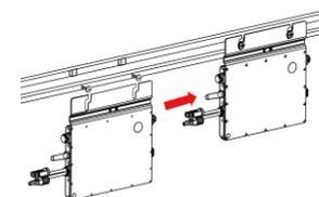
*\*Note: Please install the microinverter at least 50cm above the ground/roof for better communication with Aptos DTU.*
