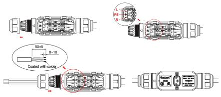
B) Connect the other side of the AC end cable to the distribution box, and wire it to the local grid network.
